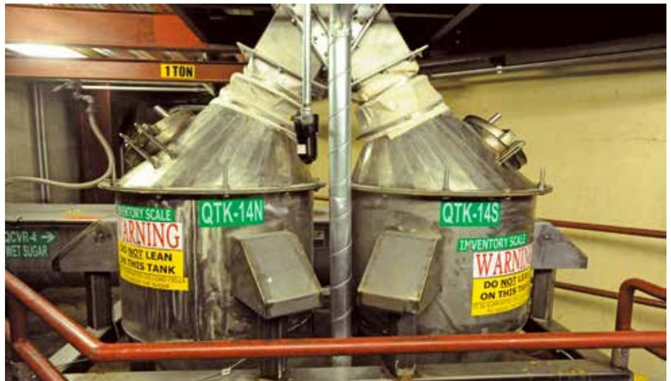
White sugar inventory scales are used to keep track of how much sugar is produced at the Twin Falls factory.
