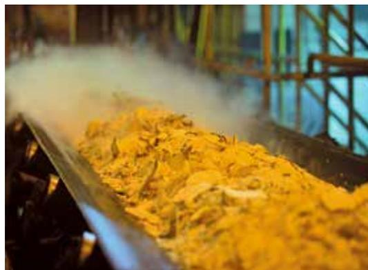
The Amalgamated Sugar Company LLC's Twin Falls factory pumps out 1,200 tons of sugar each day. Left, after sugar beets are sliced into cossettes, they go through a steamy bath.
