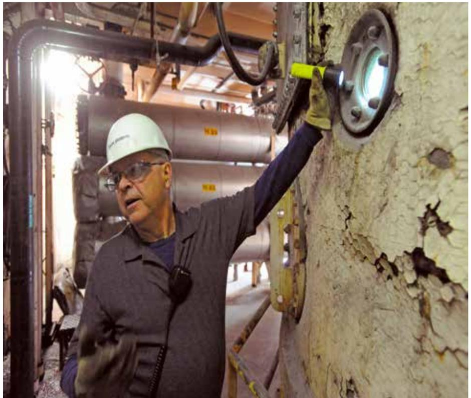
**Above: Twin Falls Production Manager Mark Branham explains how the cossettes, seen through the third-floor diffuser window, travel on to the pulp dryer. Lower left: Juice extracted from the beets is monitored every step of the way through the factory. The container at left holds juice after its second carbonation. The right container is juice after its first carbonation. Lower right: In the raw juice screen room, additional pulp is removed from the juice.**
