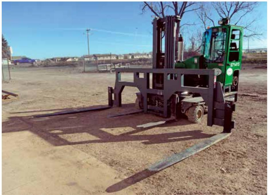
**The manufacturing division’s new Combilift simplifies moving long pieces of material in tight spaces. A special spreader bar with longer forks allows the Combi to lift a trailer and move it from bay to bay.** Rion Sanders photo
