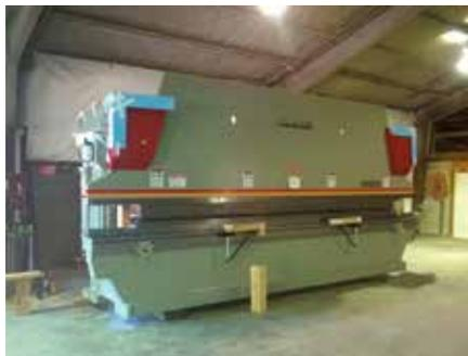
**A new press brake allows the Manufacturing Project to bend its own parts.**
