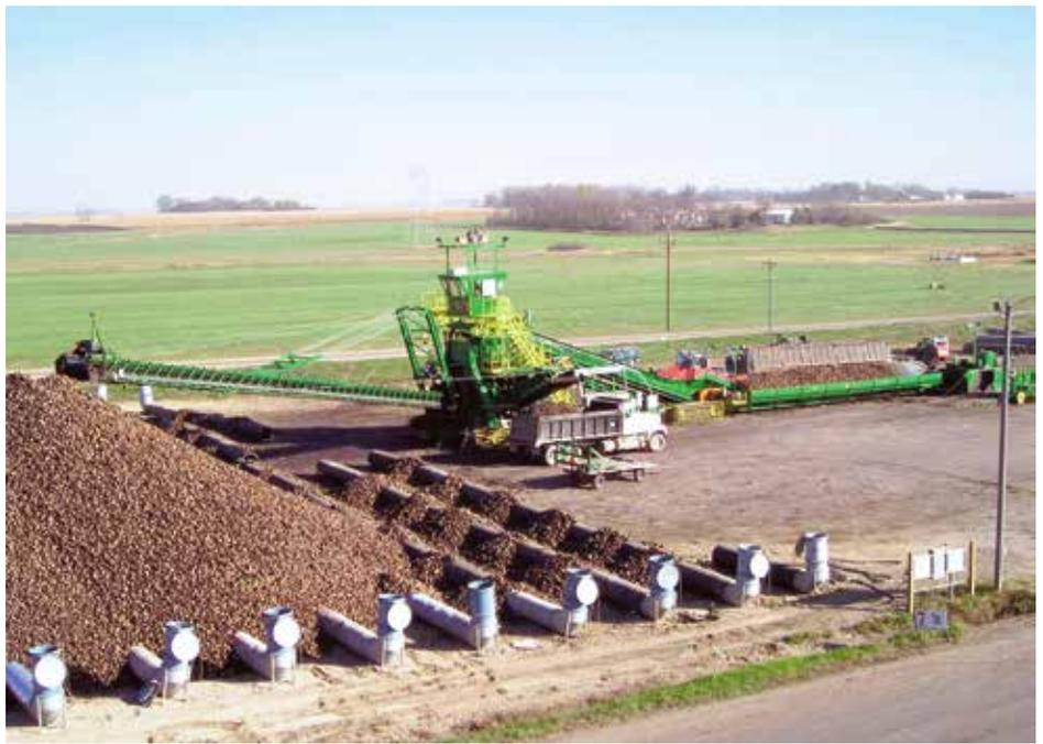
**Culverts are placed under sugar beet piles. Fans blow air through them to keep the beets cold.** Ken Dahl photo
